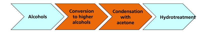
Step 2: Condensation of short-chain alcohols (e.g. ethanol)
