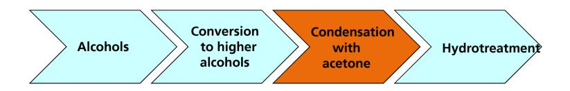
Step 3: Condensation (2:1) of received "higher" alcohols with acetone
