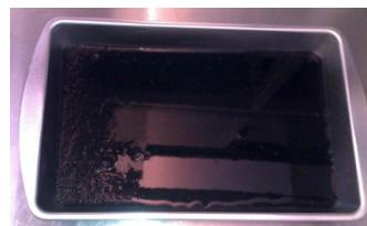
Anaerobic granular sludge from a UASB
