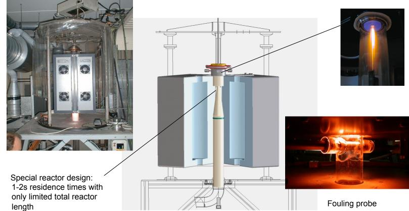
Staged gas burner: high heating rate + proper gas atmosphere
