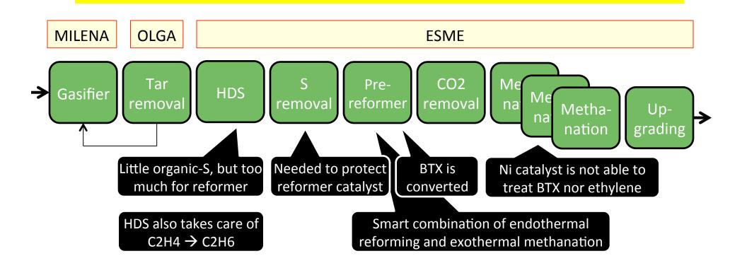
Gasifier: Fluidized Bed Gasifier operating at ~800°C
