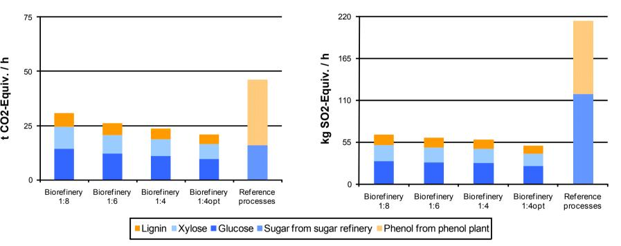
Lower CO<sub>2</sub>- and SO<sub>2</sub>- emission equivalents for the biorefinery compared to selected reference processes
