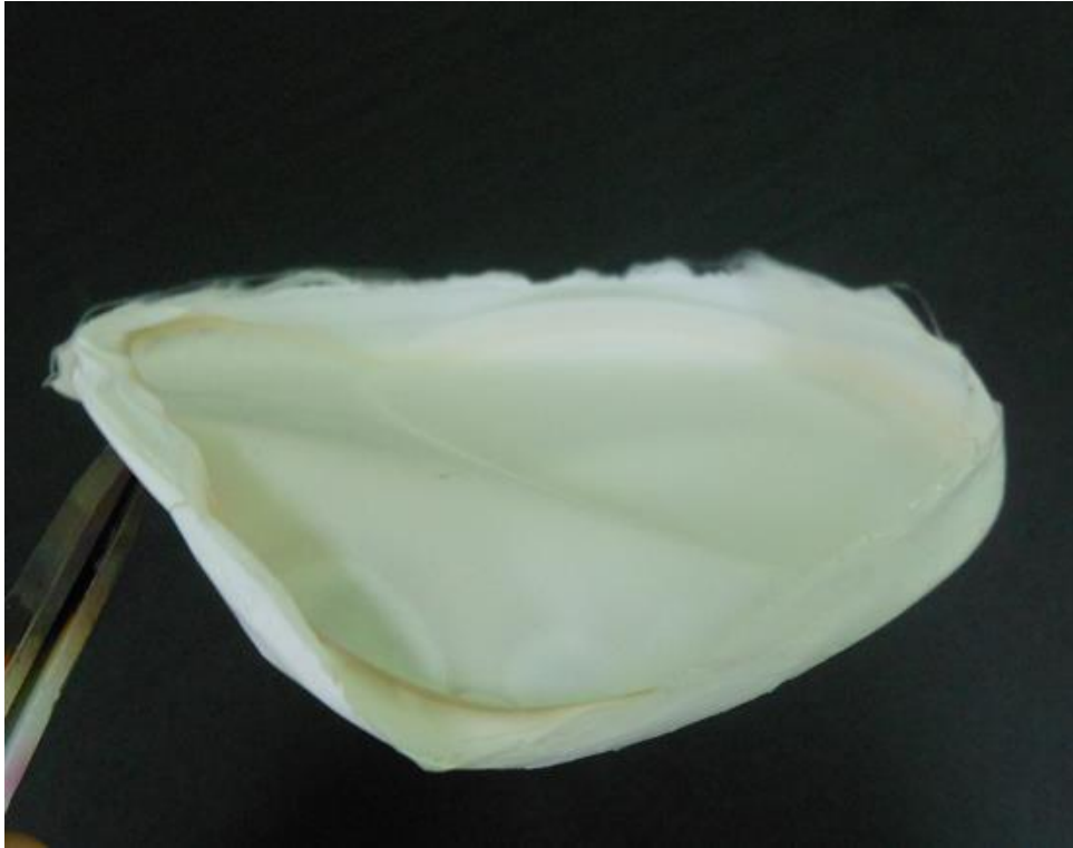
PHBV film extracted from B. xenovorans LB400 culture grown on glycerol waste and valeric acid
