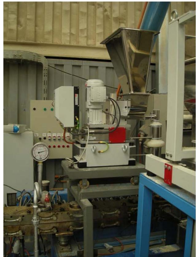
Fig. 9. Twin screw extruder TSA Industriale (L/D 40)
